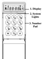
The LCD5511 shows the status of your security system using an LCD display, along with fixed symbols and numbers.
